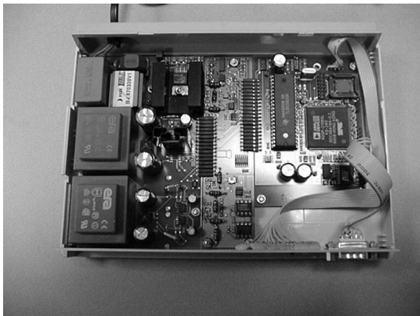
Fig. 5: Lab-prototype of OFDM-modem
